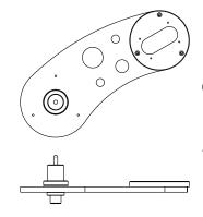
SME arm-board - pivot to spindle distance 206-240mm-- remove 6mm high Acrylic spacers - use M4x16mm bolts
