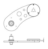
Rega arm board - pivot to spindle distance 222mm - use 6mm high Acrylic spacers - use M4x20mm bolts
