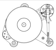
Solid and light construction of the turntable assembly has an important feature of preventing the sound-damaging resonance energy to be stored in the assembly itself.
